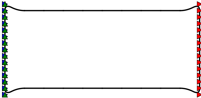
Fig. 1: Initial structure and boundary conditions. Nodes on the left edge have both degrees of freedom fixed, and nodes on the right edge have a uniform load applied horizontally.
