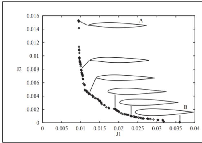
**Figure 8.9.** Optimal airfoil profiles.
